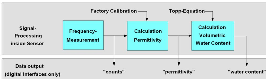
Figure 1: Signal processing chain in the sensor SMT100
